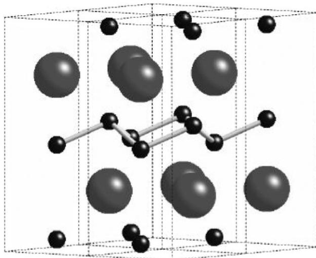
**Figure 7.** Multiple unit cells of ReB<sub>2</sub> illustrating the individual metal layers (large atoms) separated by a puckered boron network (small atoms).
