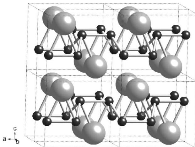
**Figure 4.** Multiple unit cells of  $\text{OsB}_2$  (osmium—large atoms, boron—small atoms) stacked on top of one another. The B–B and Os–B covalent bonds are depicted which give rise to the relatively high hardness of  $\text{OsB}_2$ .
