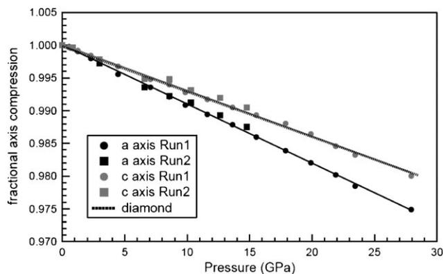
**Figure 10.** The fractional compression of ReB<sub>2</sub> separated into the *a*-axis and *c*-axis components to illustrate the anisotropic compressibility. The *a*-axis (dark symbols) is more compressible than the *c*-axis (light symbols). The *c*-axis of ReB<sub>2</sub> is as incompressible as the analogous axis of diamond (hashed line). Reproduced with permission from Ref. [62], copyright 2007 American Association for the Advancement of Science.
