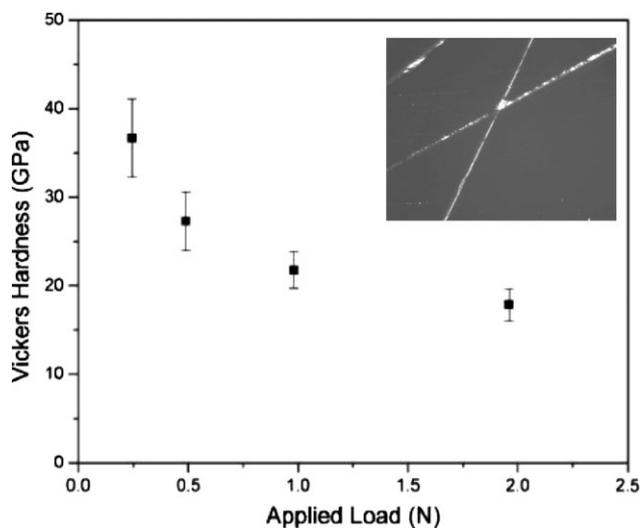
**Figure 6.** Vickers hardness of  $\text{OsB}_2$ , possessing a maximum hardness of 37 GPa. Inset: sapphire window scratched by  $\text{OsB}_2$  powder viewed under  $500\times$  magnification in an optical microscope. Adapted with permission from Ref. [50], copyright 2008 Materials Research Society.
