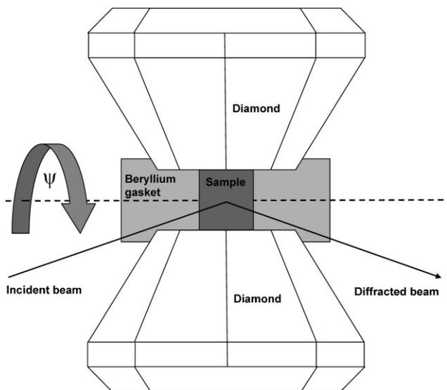
**Figure 3.** Radial diffraction geometry for high pressure experiments. The cell is rotated about the axis  $\psi$ , and data are collected through the gasket rather than through the diamonds as in conventional DAC experiments.
