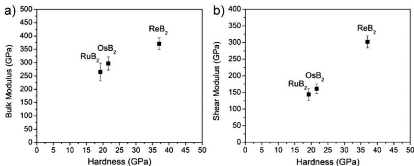
**Figure 12.** Hardness plotted as a function of bulk modulus (left) and shear modulus (right) illustrating the better correlation between hardness and shear modulus. Reprinted with permission from Ref. [19], copyright 2008 American Institute of Physics.
