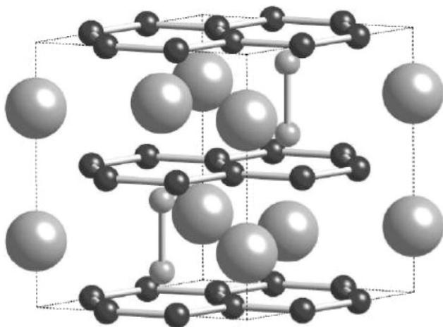
**Figure 13.** The crystal structure of  $WB_4$ . The boron atoms (small atoms) form a hexagonal network in addition to covalent dimers that result in a 3-dimensional network. The tungsten atoms (large atoms) form hexagonal layers in between the boron sheets.
