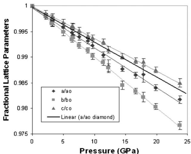
**Figure 5.** Comparison of the compressibility of the individual lattice parameters of  $\text{OsB}_2$  with diamond. The  $a$  ( $\blacklozenge$ ),  $b$  ( $\blacksquare$ ), and  $c$  ( $\blacktriangle$ ) parameters in  $\text{OsB}_2$  are fit with straight lines. Note that the  $c$ -axis in  $\text{OsB}_2$  is less compressible than the analogous axis of diamond. Reproduced with permission from Ref. [46], copyright 2005 American Chemical Society.
