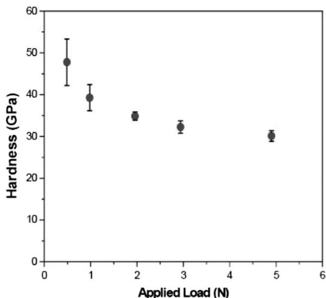
**Figure 8.** The Vickers hardness of  $\text{ReB}_2$  is plotted as a function of applied load. The average hardness increases from 30 to 48 GPa as the applied load decreases from 4.9 to 0.49 N. Reproduced with permission from Ref. [62], copyright 2007 American Association for the Advancement of Science.
